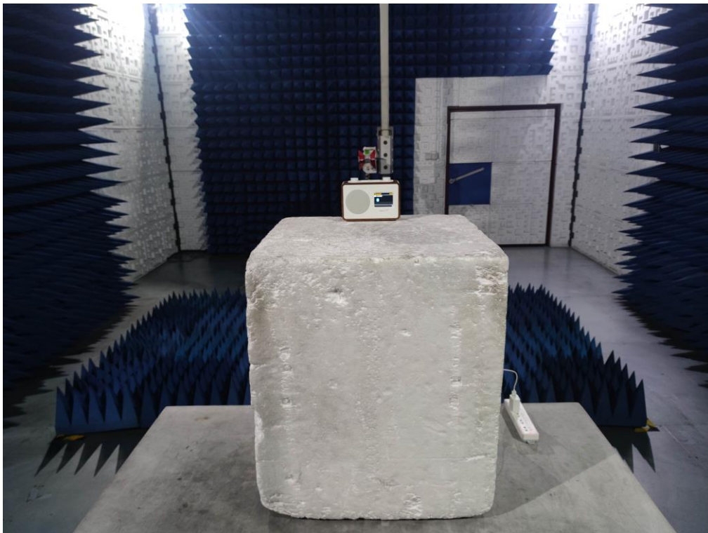
RADIATED EMISSION TEST SETUP ABOVE 1GHz
