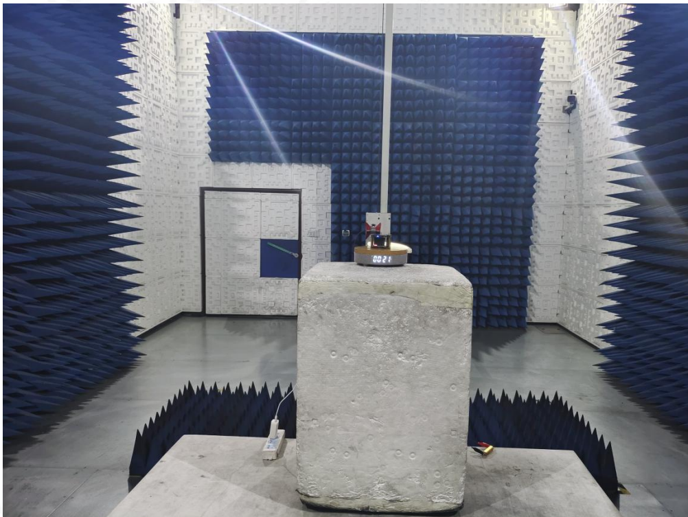
RADIATED EMISSION TEST SETUP ABOVE 1GHZ
