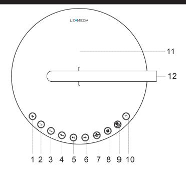
1.  $\circlearrowleft$ /**M** [Standby/ MODE]: Plug in the mains power or switch the power switch "ON" position at the rear panel to power on the DTS2 unit and enter Soothing sleep music automatically. Briefly Press M to switch FM mode, Bluetooth mode and Soothing music mode in turn.
