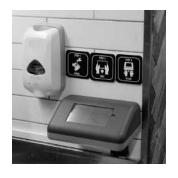
13. Position the Wash, Dry, Scan tiles above or next to the Hand Scanner to help communicate process to users.
