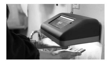
If the light turns on when you place your hands beneath the Hand Scanner, then you have successfully mounted your Hand Scanner.
