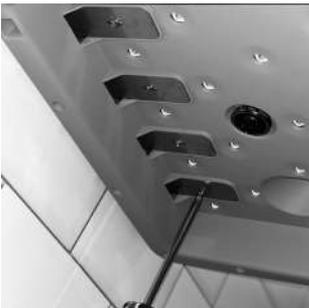
12. Tighten the bolts up into the bracket through the holes visible on the bottom of the device.
