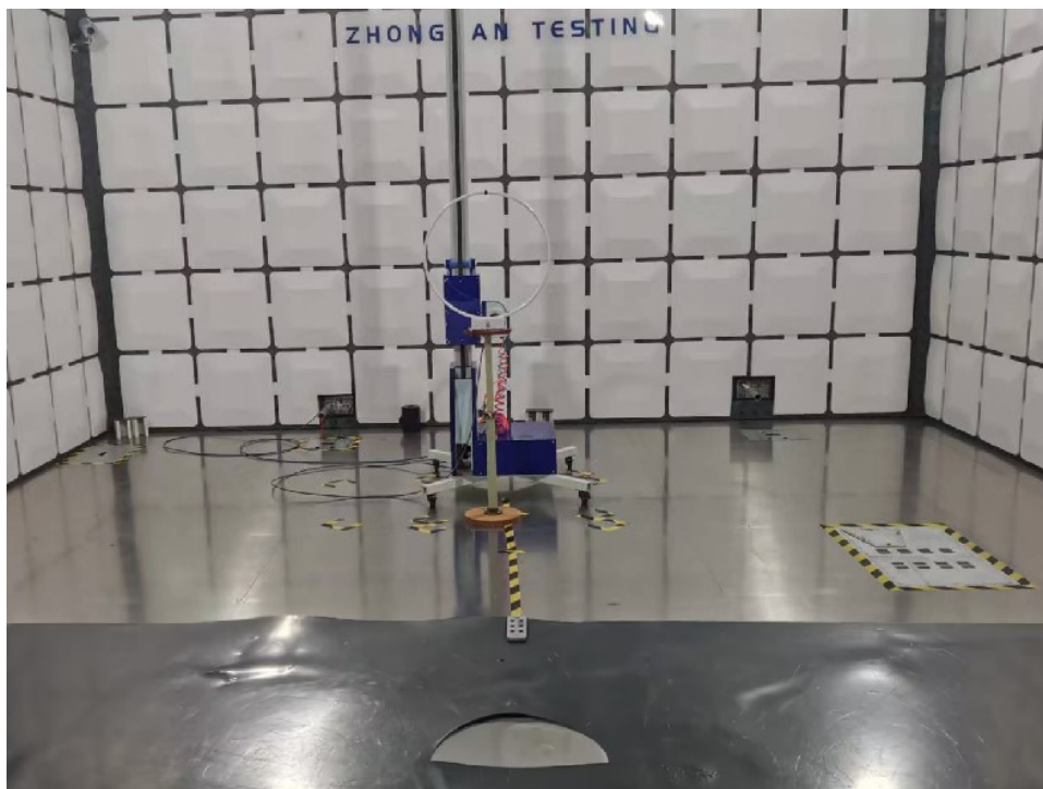
Photograph 1: Set-up for Radiated Spurious Emission, 9kHz - 30MHz
