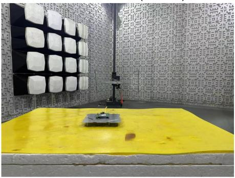
Transmitter Radiated Unwanted Emissions(Above 1GHz)
