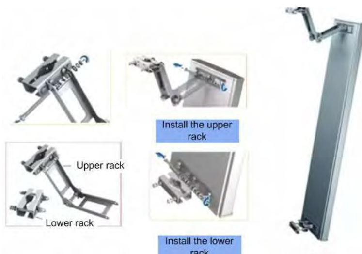
Figure 3-11 Installer Assembling Procedure of Directional Antennas
