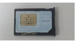
Step 2 insert the SIM metal face up and into the holder with the missing end facing the outside. Then push the card holder into the card slot:
