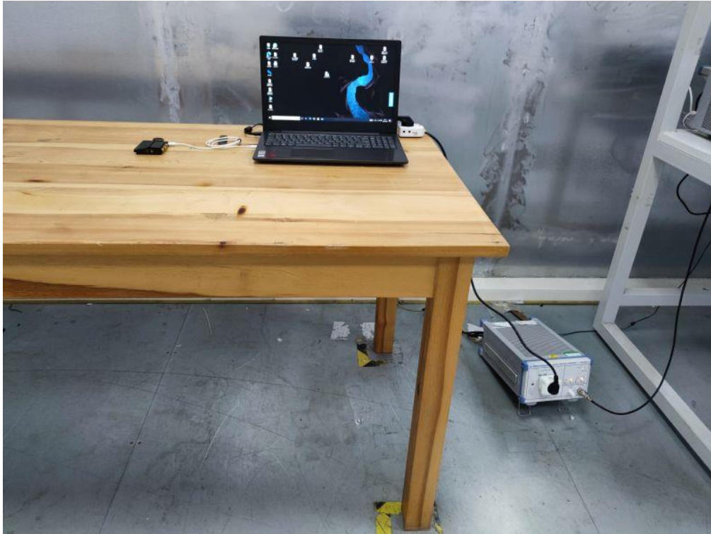
Photo of Power Line Conducted Measurement
