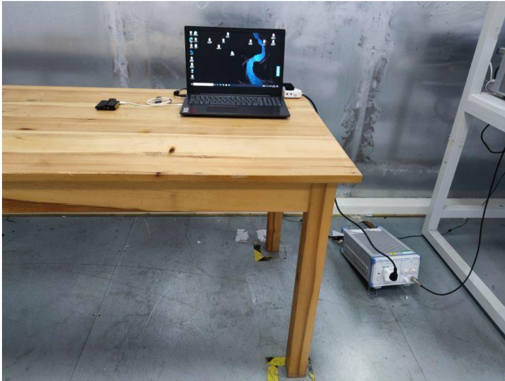
Photo of Power Line Conducted Measurement
