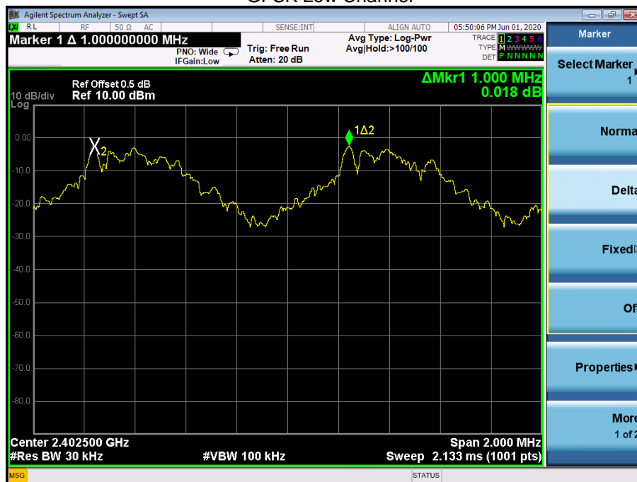
Test plots GFSK Low Channel
