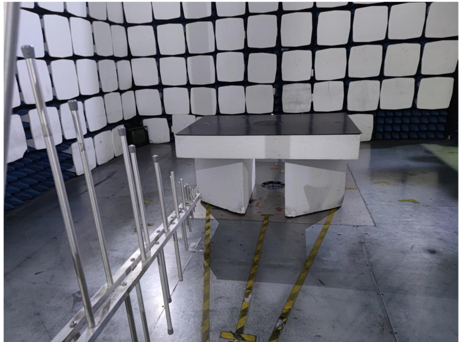
Radiation Emission Test Setup (30MHz to 1GHz)
