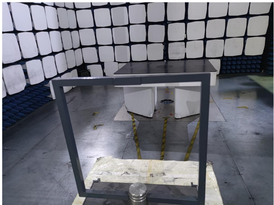
Radiation Emission Test Setup (Below 30MHz)
