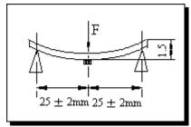
Weld the product to the center part of the PCB with the thickness  $1.6\pm0.2$ mm as the illustration shows, and keep exerting force arrow-w ard on it at speed of :1mm/S, and hold for  $5\pm1$ S at the position of 1.5mm bending distance, so far, any peeling off of the
