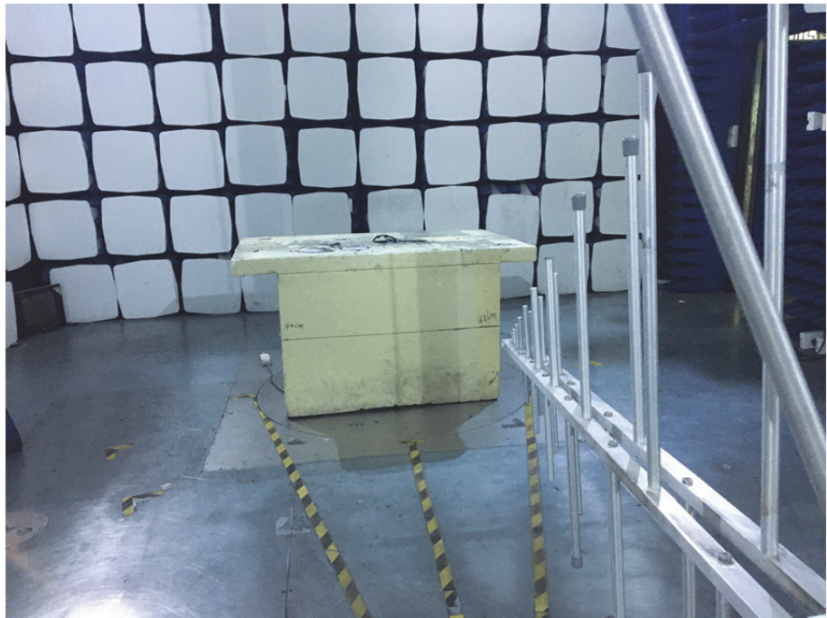
Radiation Emission Test Setup (30MHz to 1GHz)
