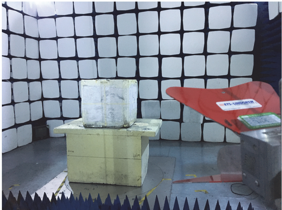
Radiation Emission Test Setup (1GHz to 18GHz)
