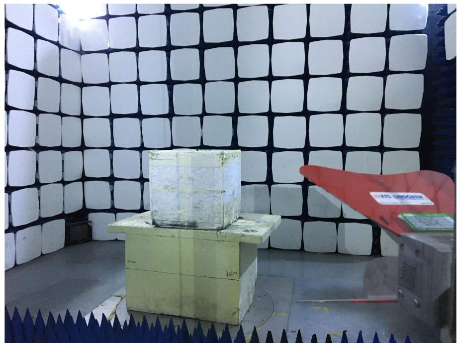
Radiation Emission Test Setup (1GHz to 18GHz)
