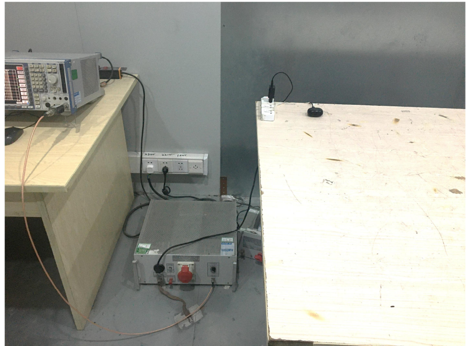
Conducted Emission Test Setup
