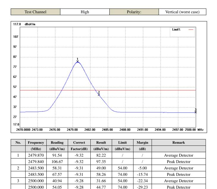
*Note: Average measurement was not performed if peak level is lower than average limit(54 dBuV/m) for above 1GHz.*
