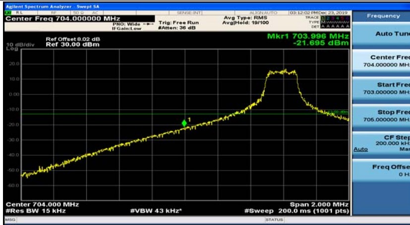
Channel Bandwidth: 10 MHz_LCH_16QAM_1RB#24
