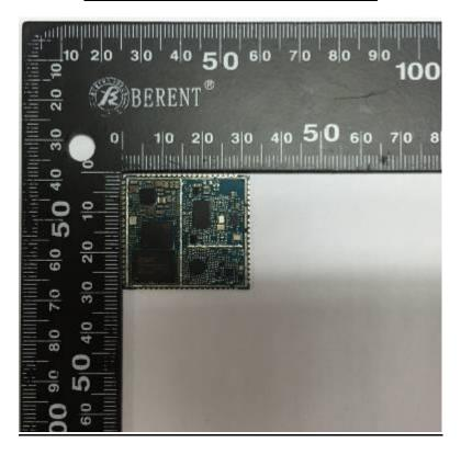
**EUT- Top Shielding Cover off Zoom in View**
