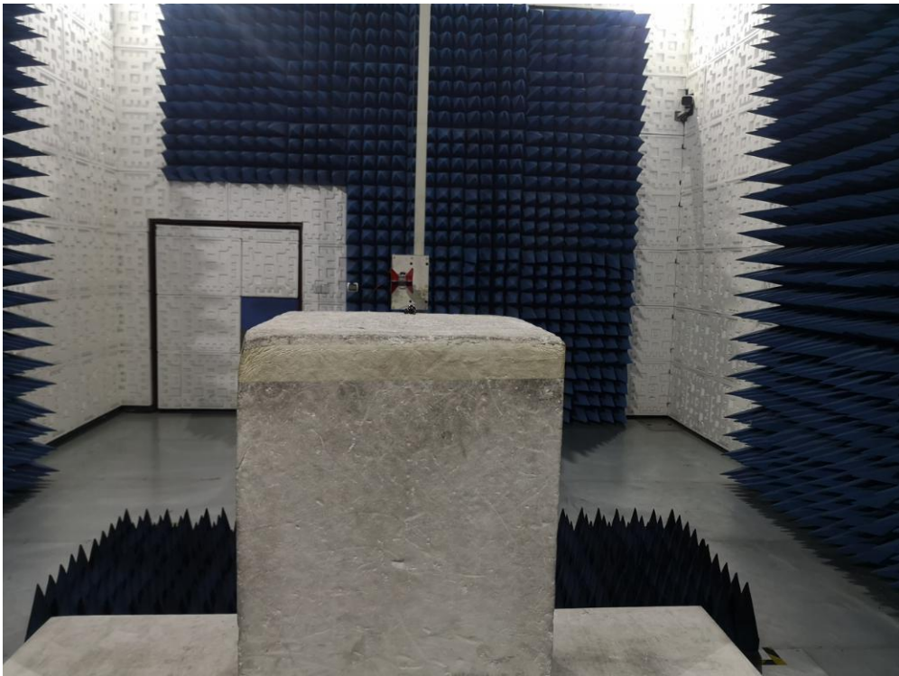
RADIATED EMISSION TEST SETUP ABOVE 1GHz
