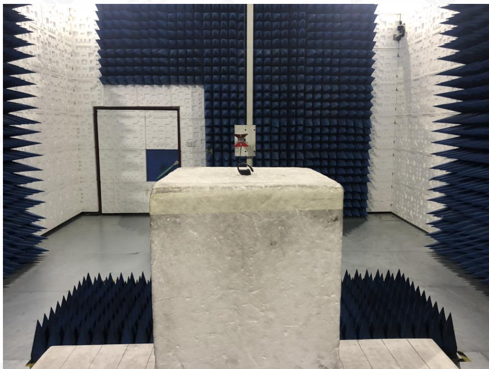
RADIATED EMISSION TEST SETUP ABOVE 1GHZ
