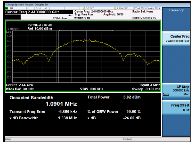
GFSK (BLE 1Mbps) MIDDLE CHANNEL
