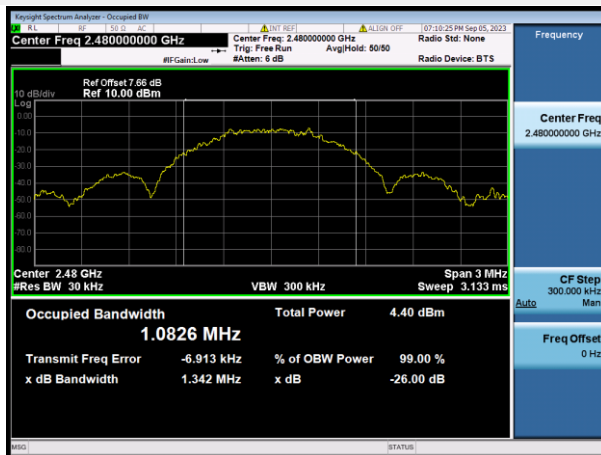
GFSK (BLE 1Mbps) HIGH CHANNEL
