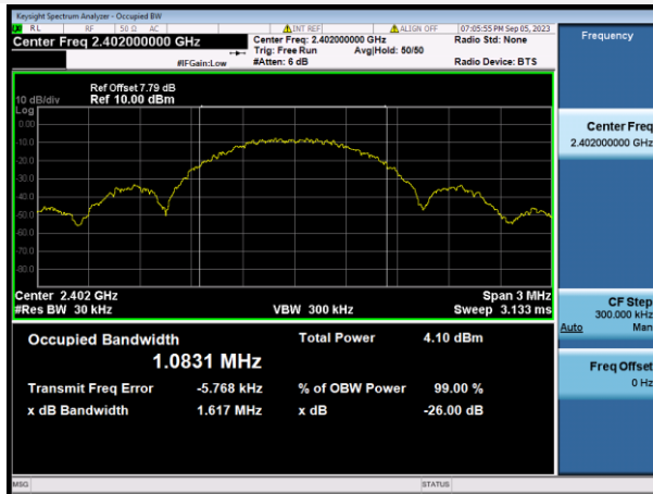
GFSK (BLE 1Mbps) LOW CHANNEL
