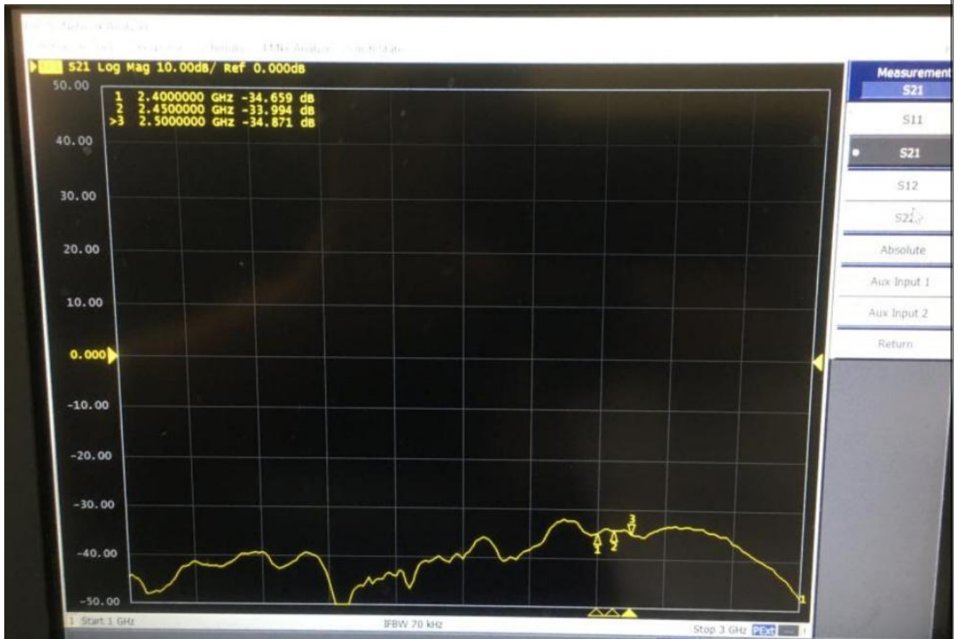
WiFi and BT antenna isolation data (about -33~-34dB)
