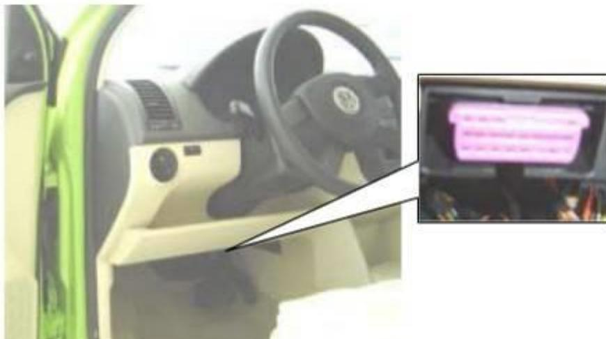
\*VW POLO: the OBD plug is below the dashboard, use SMART OBDII-16 connector.
