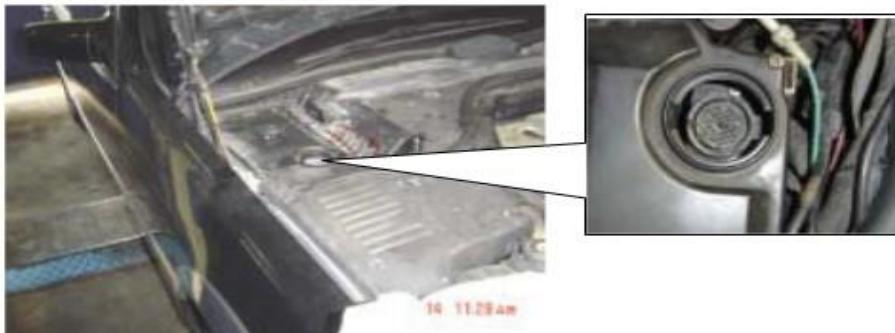
\*Benz 300SEL 140 chassis: the OBD plug is on the left hand side of the engine bay, use Benz-38 connector.
