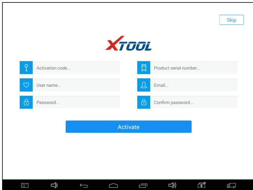
**1.2.** Input activation code (on the Quality Certificate cover), product serial number (each device will have a serial number and activation code), nickname (workshop's name or user's nickname), login account (can be your email address or cell phone number) and password, the system will then save it. Activation is a one time process. The diagnostic application will start after activation.
