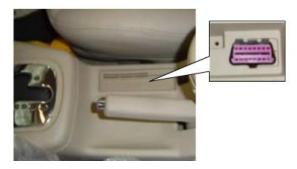
\*VW Passat B5: the OBD plug is behind the gearlever and beside the parking brake lever. It will appear when take away the cover. we can use SMART OBDII-16 connector.
