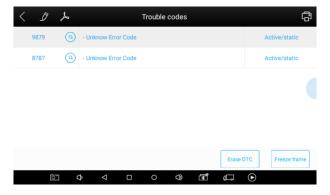
Tip: In the process of diagnosis, if the device shows "System is OK" or "No Trouble Code", it means there is no related trouble code stored in ECU or some troubles are not under the control of ECU, most of these troubles are mechanical system troubles or executive circuit troubles, it is also possible that signal of the sensor may bias within limits, which can be judged in Live Data.
