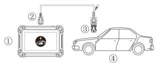
① PS70PRO Mainframe ② Main Test Cable ③ OBD II -16 ④ Vehicle
