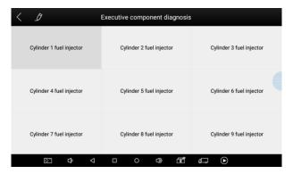
Tip: **Actuating Components Test** performs function tests for parts of system actuating components. When performing this function, the diagnostic tool will take action test by simulating ECU signal to judge whether the actuating components or circuits are good.
