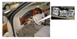
\*GM Buick: the OBD plug is below the dashboard,we can use SMART OBDII-16 connector.
