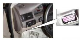
\*AUDI A6: the OBD plug is on the lower left side of the dashboard, we can use SMART OBDII-16 connector.
