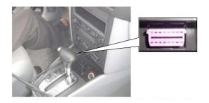
\*VW Bollywood 1.8: the OBD plug is below the console, we can use SMART OBDII-16 connector.
