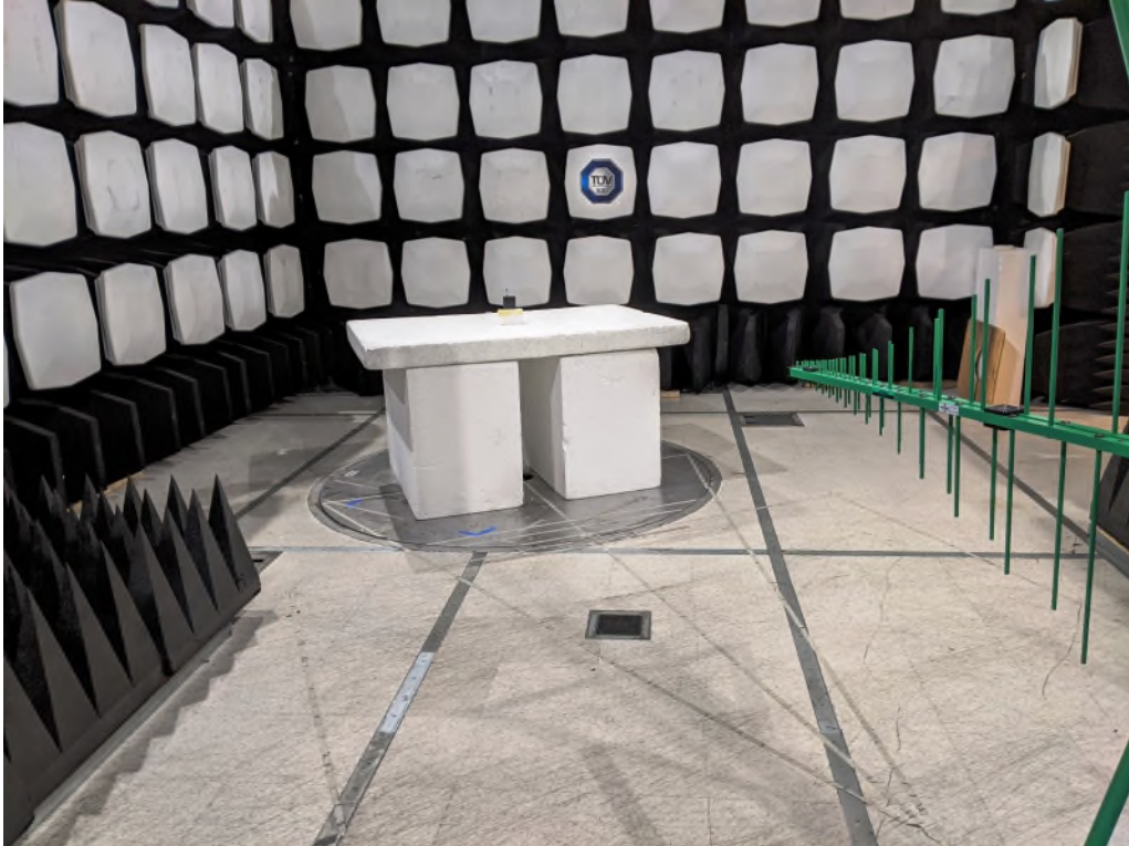
Figure 8: Equipment Under Test – Radiated Emissions <1GHz
