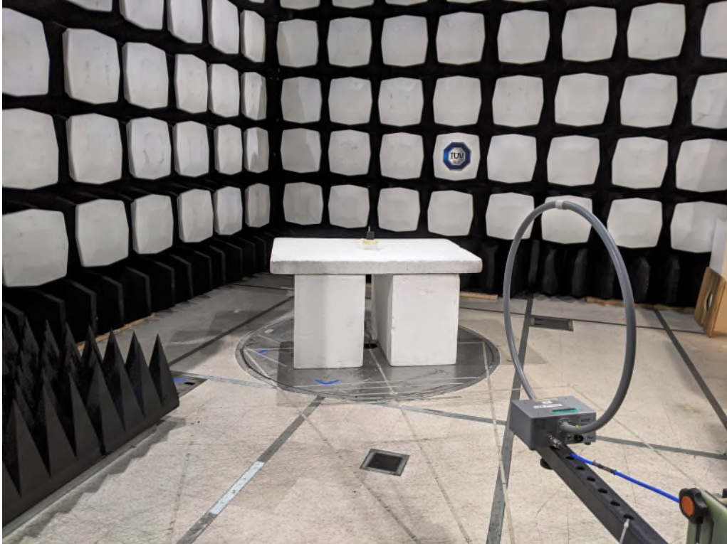
Figure 6: Equipment Under Test – Radiated Emissions <30MHz
