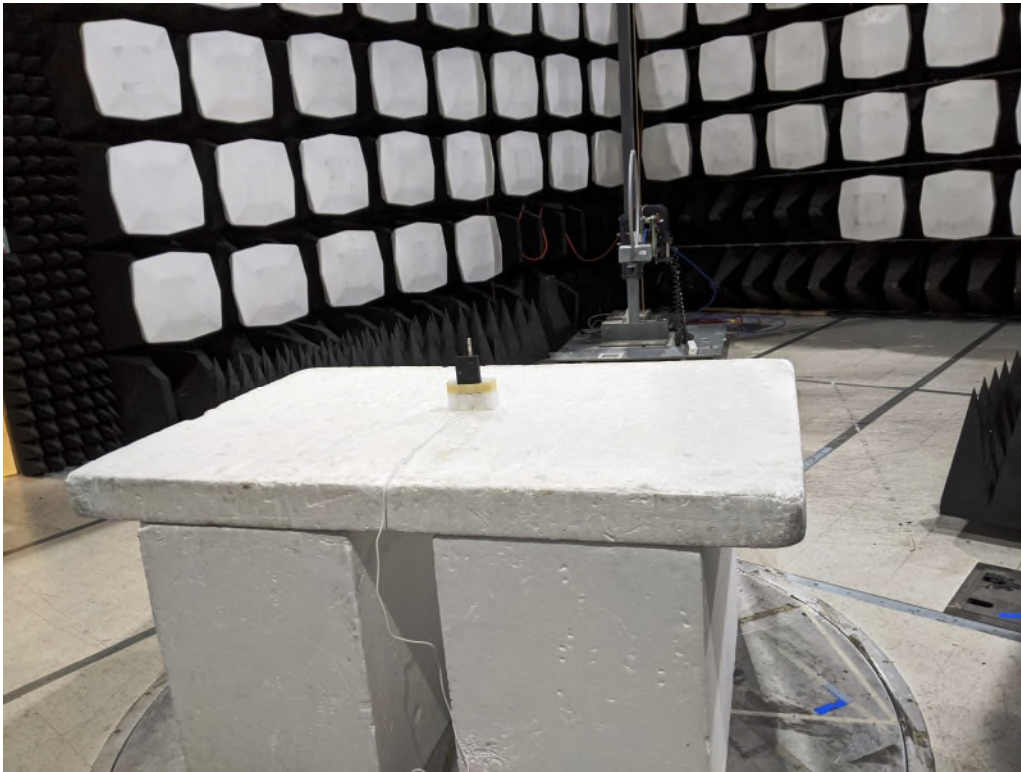
Figure 7: Equipment Under Test – Radiated Emissions <30MHz
