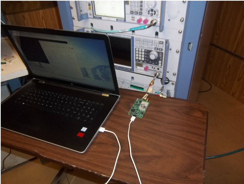
Figure 1: Equipment Under Test – Antenna Port Conducted Measurements (Unlicensed)
