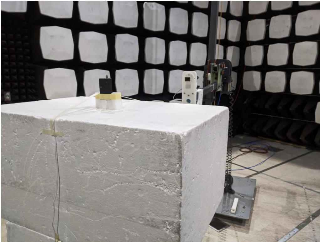
Figure 13: Equipment Under Test – Radiated Emissions >18GHz
