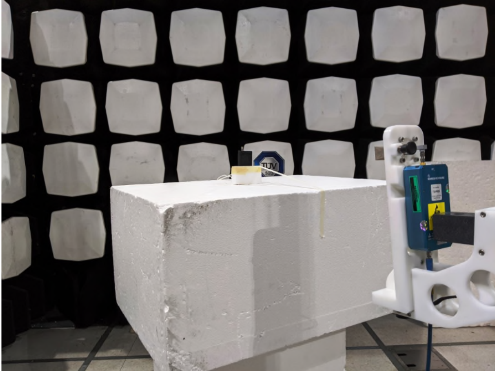
Figure 12: Equipment Under Test – Radiated Emissions >18GHz
