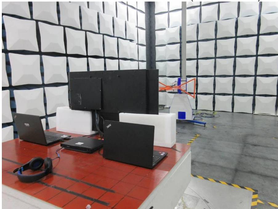
RADIATED RF MEASUREMENT SETUP (30MHz ~ 1 GHz)
