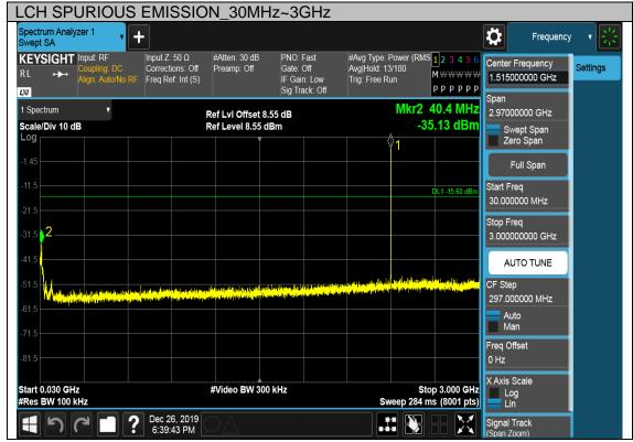
Note: The point 1 which exceeds the limit is 2.4G main carrier.
