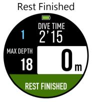
Dive Depth 1m-30m (3ft - 100ft) Notify user when the Surface Time reaches 2 times of the dive time of last dive.
