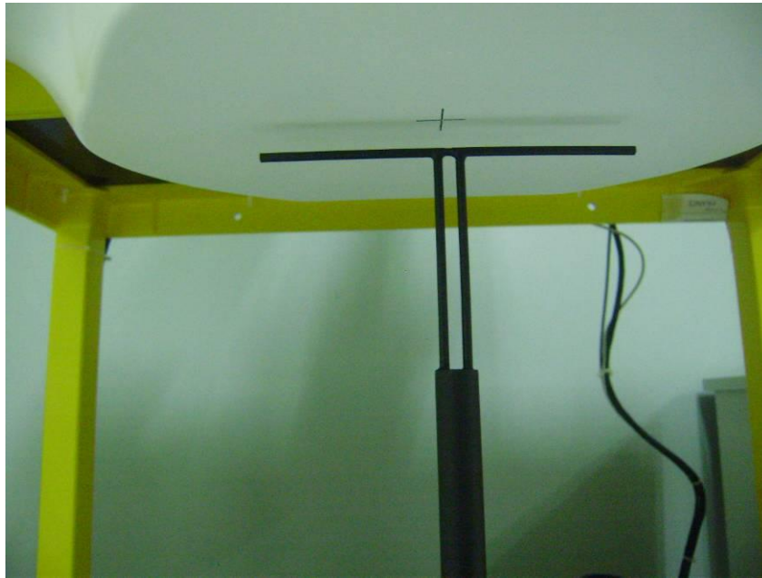
Fig 6.2 Setup Photo of Dipole Antenna
