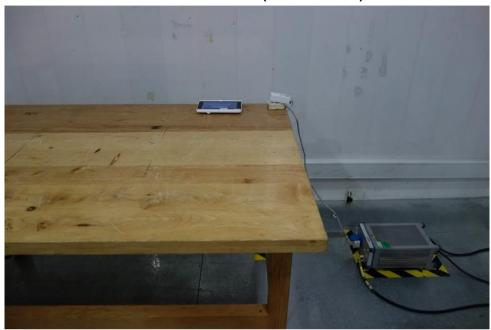
Field Strength of the Fundamental Signal (15.231(b))
