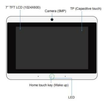
LCD: 7" TFT LCD (1024X600)
