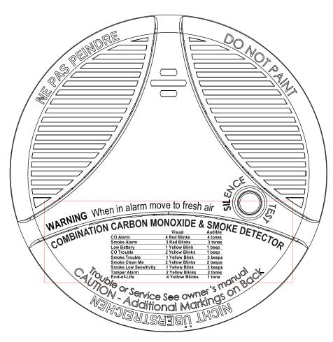
LABEL. e Laser printing area H 31mm W 94mm WARNING When in alarm move to fresh air
