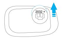
6. Slide a new CR2032 battery into the battery casing, making sure that the polarity is correct.
