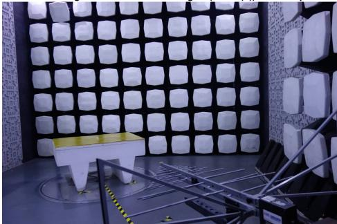
1.2 Radiated Emissions Test Setup
