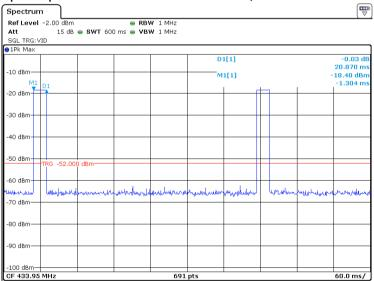
The duty cycle is simply the on-time divided by the observation time:
