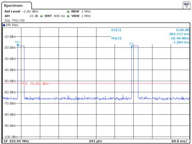
The pulse period is exceeded 0.1 seconds, so the observation time is 100ms.
