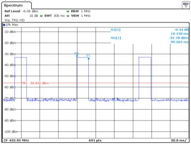
The duty cycle is simply the on-time divided by the observation time:
