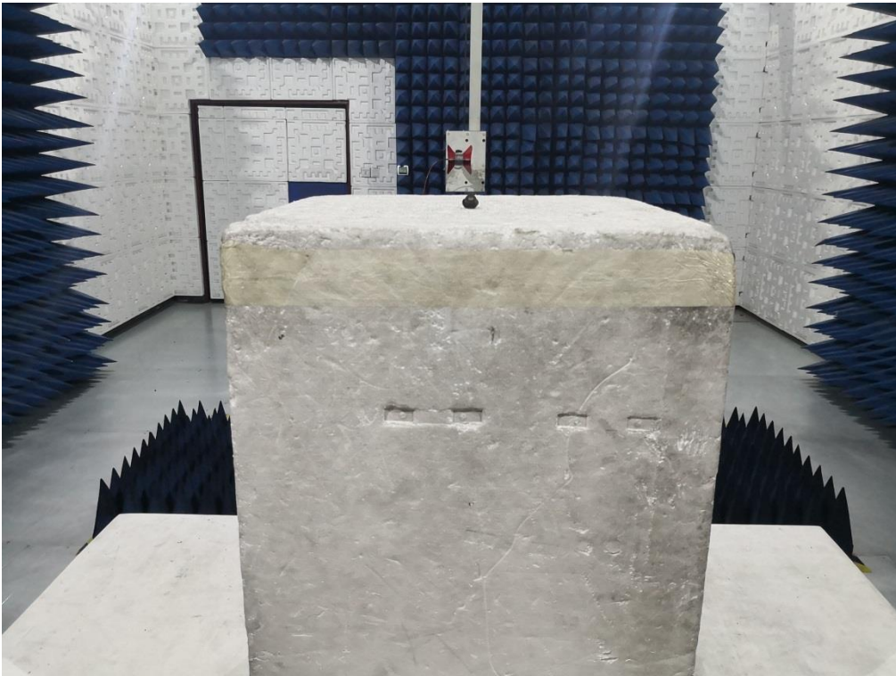
RADIATED EMISSION TEST SETUP ABOVE 1GHz
