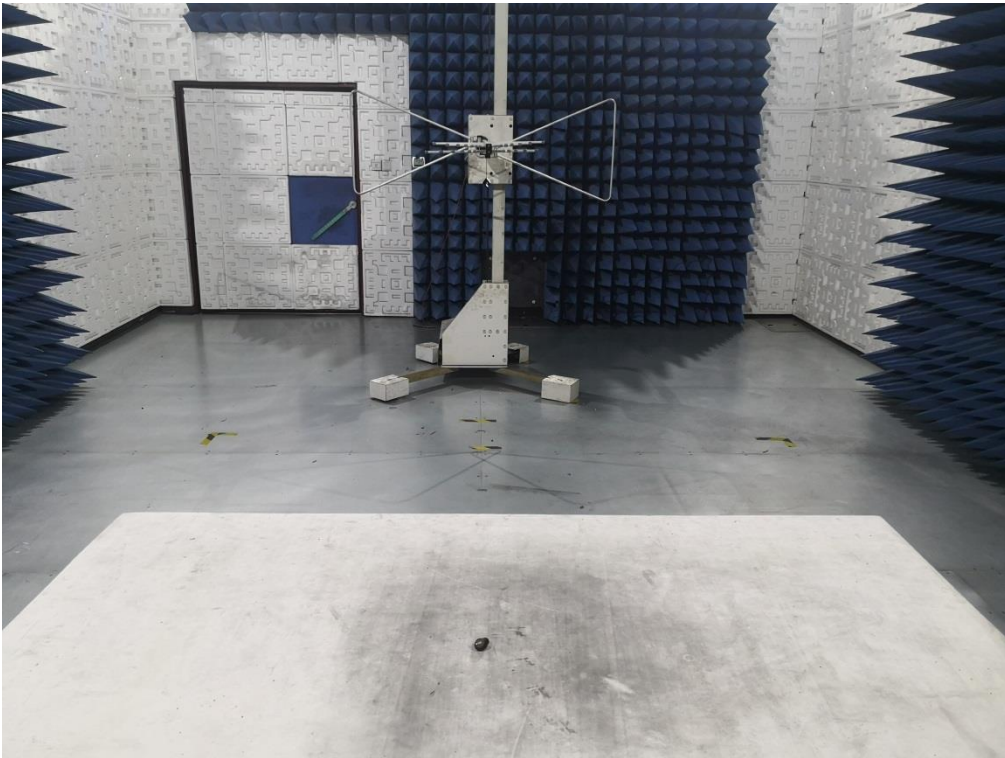
RADIATED EMISSION TEST SETUP ABOVE 1GHz
