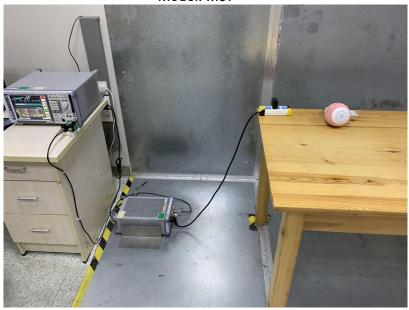
Radiated Spurious Emissions From 30MHz-1000MHz
