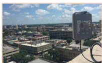
Point-to-Point Broadband Next generation point-to-point broadband links over 2Gb/s, 1 mile, under $200 per node
