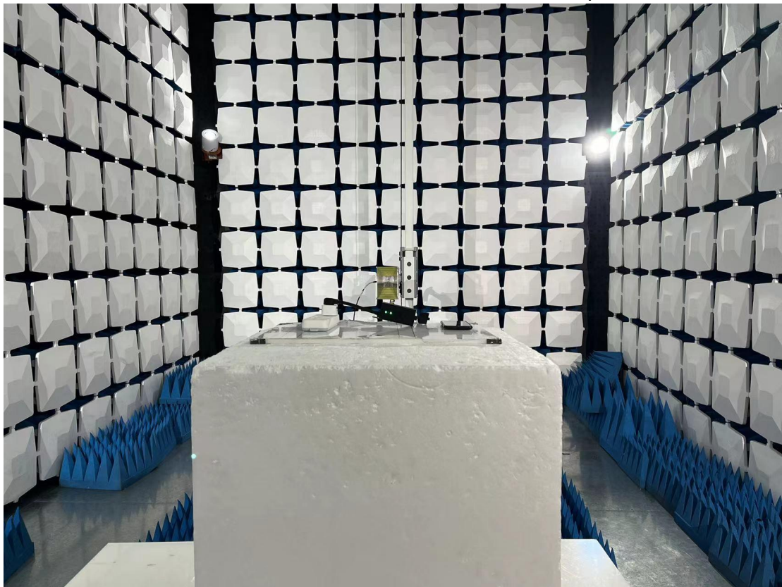
Above 1GHz for radiated emission test setup
