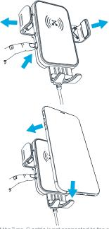
NOTE: if the Type-C cable is not connected to the charger, the clamps will not close automatically. You will need to press the lateral button to close them to hold your phone. When the power is off, it will beep as a reminder to take the phone away.
