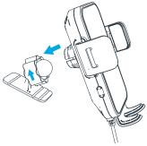
Attach the charger's mount onto the dash mount and turn the adaptor to tighten and secure it.
