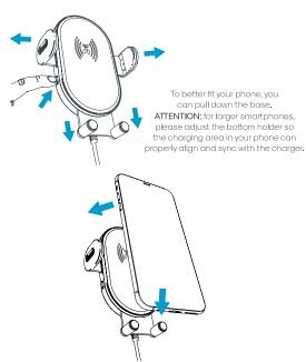
NOTE: if the Type-C cable is not connected to the charger, the clamps will not close automatically. You will need to press the lateral button to close the clamps around your phone. When the power is off, it will beep 5 times to remind you to take away the phone.
