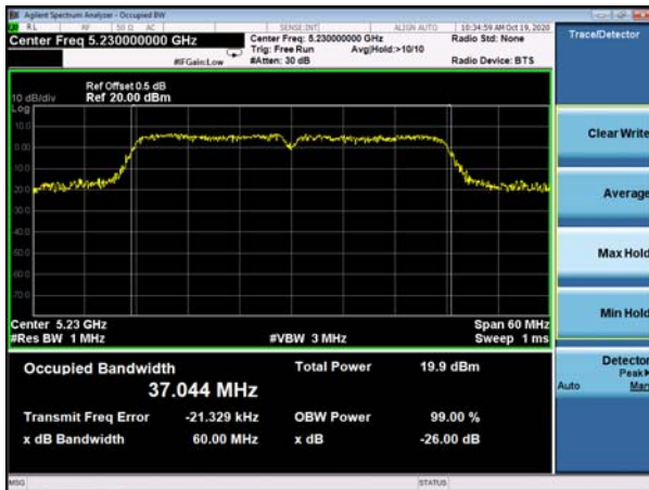
(802.11 n40) 26dB&99%Bandwidth plot on channel 46
