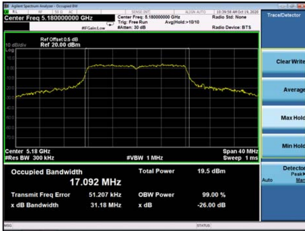
(802.11a) 26dB&99%Bandwidth plot on channel 40
