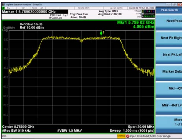
(802.11a) PSD plot on channel 165
