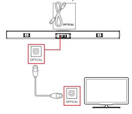
Note: please refer to the fiber output equipment manual to switch the output equipment to fiber mode.
