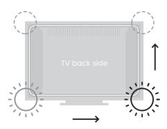
The light spot will blink indicating that the Lightpack remembered the corner position. Then the spot will continue moving.
