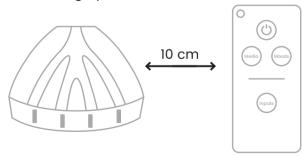
**4.** When connected, the Remote will blink on and off.
