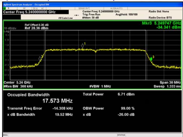
(802.11 n20) 26dB Bandwidth plot on channel 48
