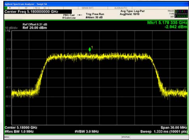
(802.11n20) PSD plot on channel 36
