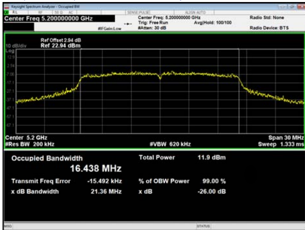
(802.11a) 99% Bandwidth plot on channel 40
