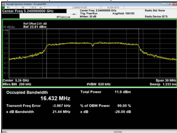
(802.11ac20) 99% Bandwidth plot on channel 48
