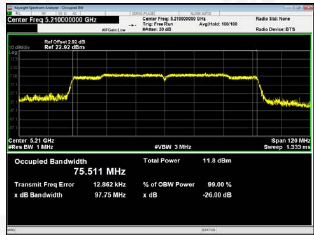
(802.11 ac80) 99% Bandwidth plot on channel 42
