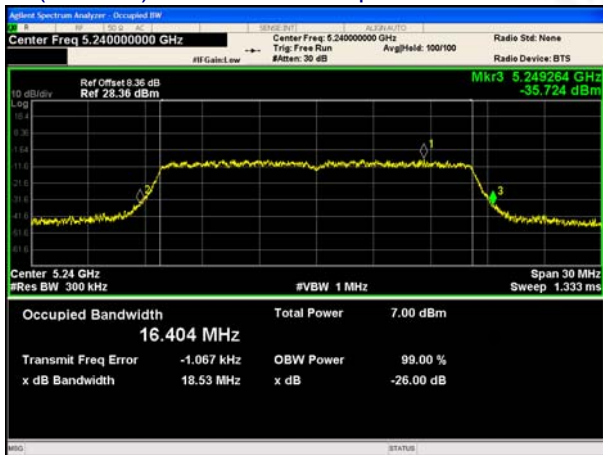
(802.11a) 26dB Bandwidth plot on channel 48
