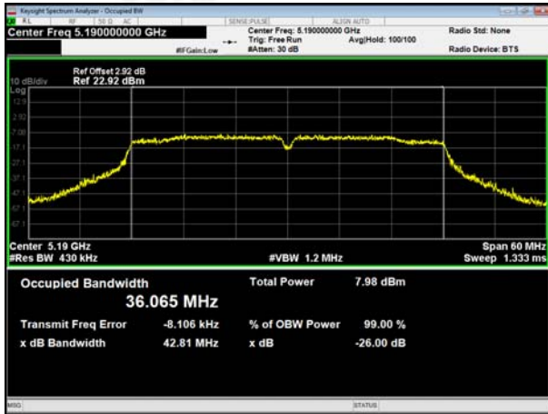
(802.11 n40) 26dB Bandwidth plot on channel 46
