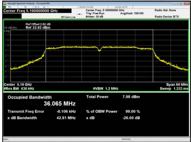
(802.11 ac40) 26dB Bandwidth plot on channel 38
