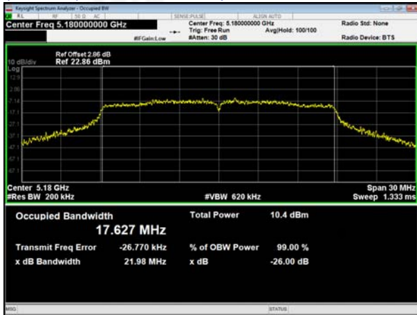
(802.11a) 99% Bandwidth plot on channel 36
