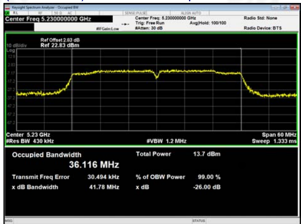
(802.11 ac40) 26dB Bandwidth plot on channel 46
