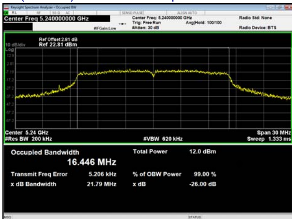
(802.11a) 99% Bandwidth plot on channel 48
