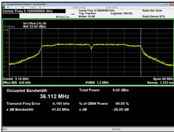
(802.11 n40) 99% Bandwidth plot on channel 38
