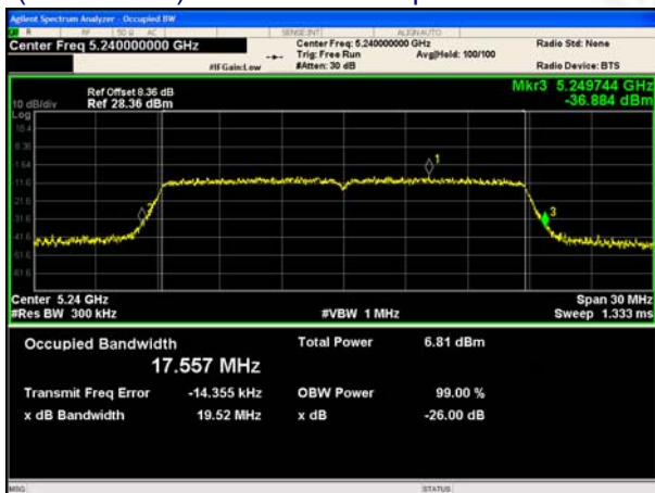
(802.11ac20) 26dB Bandwidth plot on channel 48
