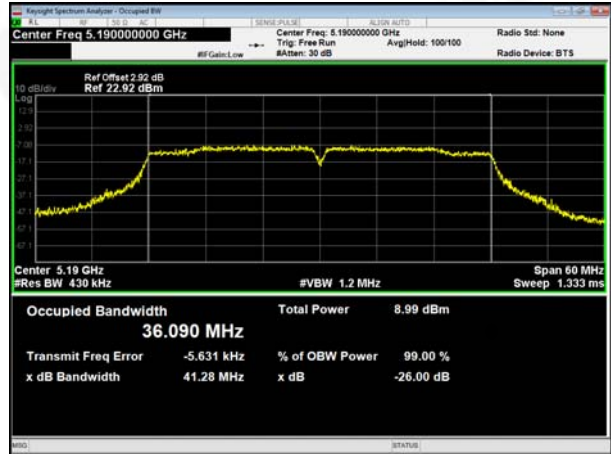
(802.11 ac40) 99% Bandwidth plot on channel 38
