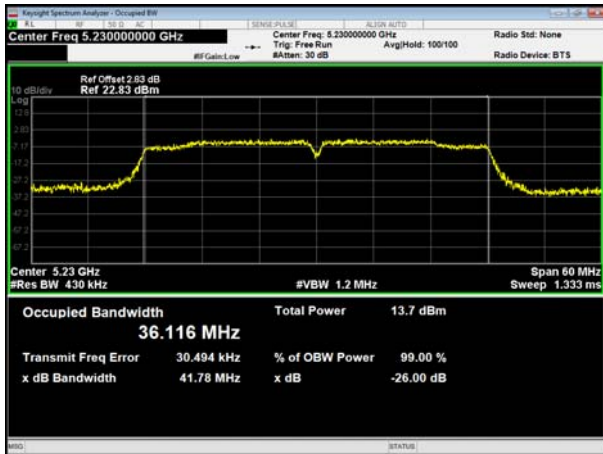
(802.11 n40) 26dB Bandwidth plot on channel 46
