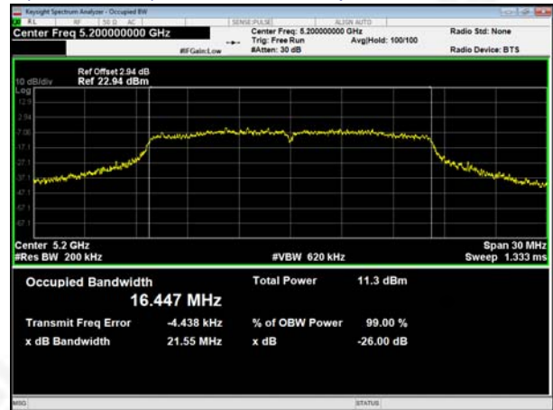
(802.11 n20) 99% Bandwidth plot on channel 40
