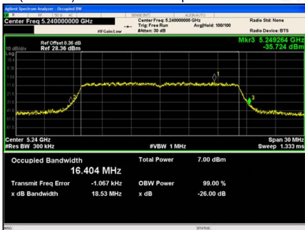
(802.11a) 26dB Bandwidth plot on channel 48
