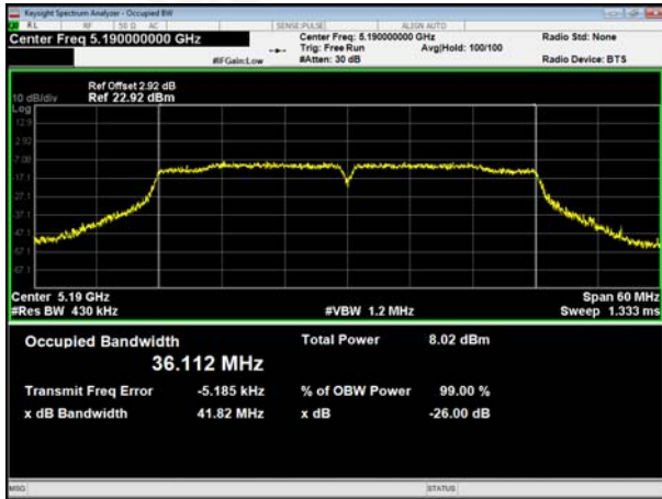
(802.11 n40) 99% Bandwidth plot on channel 38
