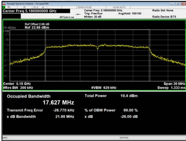
(802.11a) 99% Bandwidth plot on channel 36
