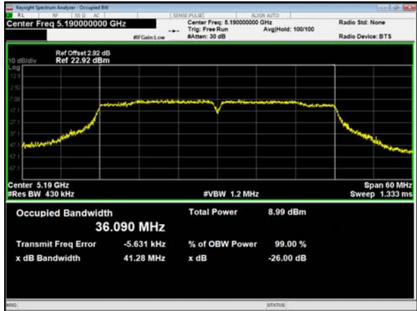
(802.11 ac40) 99% Bandwidth plot on channel 38
