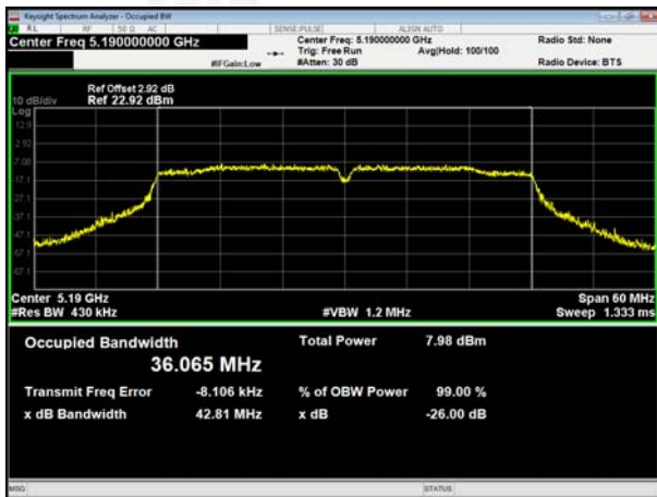
(802.11 n40) 26dB Bandwidth plot on channel 38
