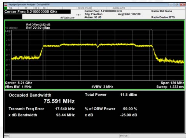
(802.11 ac80) 26dB Bandwidth plot on channel 42
